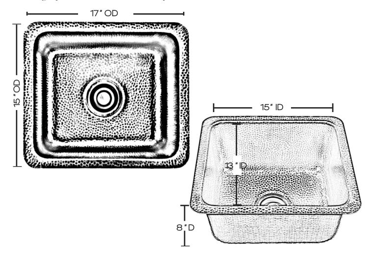
Your copper sink is handmade and therefore a work of art. Each sink is unique and can vary 1/4" in either direction. We highly recommend waiting to receive your sink before cutting your counter top.
